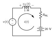
Find the transfer function,  $V_L(s)/V(s)$ , for the electrical network shown in Fig., which contains a nonlinear resistor whose voltage-current relationship is defined by  $i_r=2e^{0.1v_r}$ , where  $i_r$  and  $v_r$  are the resistor current and voltage, respectively. Also, v(t) in Fig is a small-signal source.
