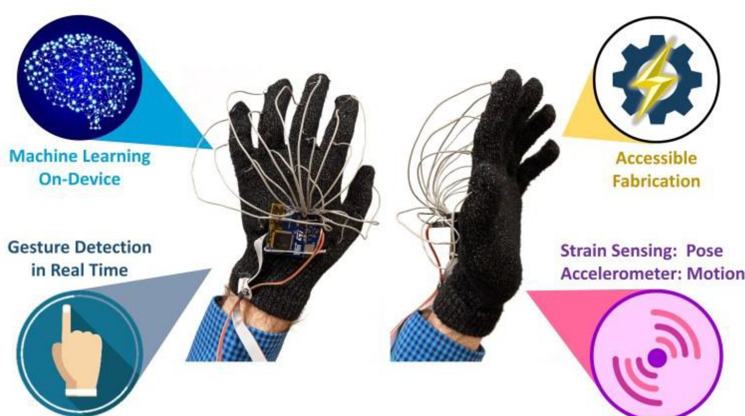
Figure 1. Overview of the Smart Glove System for Gesture Recognition [1]
