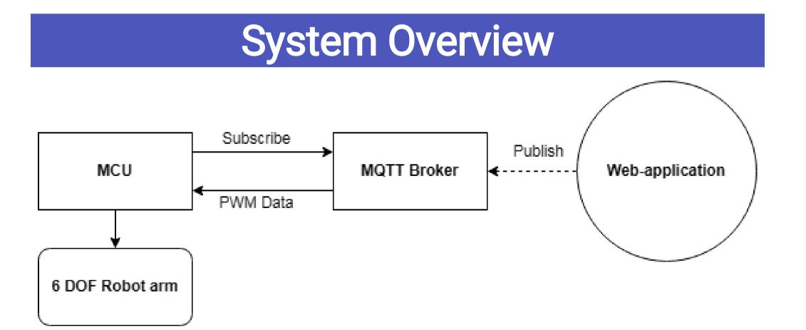
The MQTT broker is used to efficiently manage message distribution and state synchronization across the network, enabling real-time control and monitoring of IoT devices. The system features a dynamic web application operated sliders. The 3D scene using WebGL dynamically renders models such as a robotic arm that can be manipulated in real-time, reflecting changes from user inputs and physical simulations.
