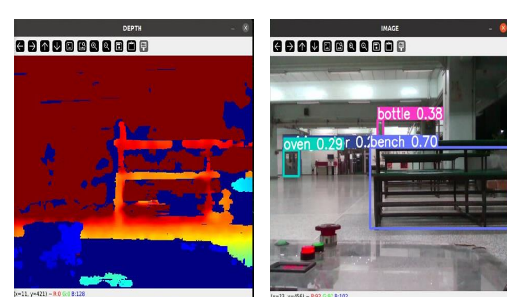
Figure 6 : Distance Estimation and Object Detection with Yolov5s
