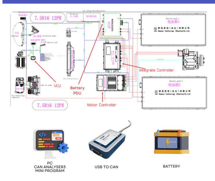
Connecting wire and communication cables to systems and components. We use a CAN analyzer to connect to the communication line to read CAN bus message.
