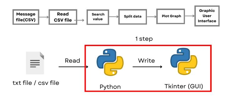
We use python to analyze data from CAN bus messages. Then using tkinter to create Graphic User Interface for display values and graph.
