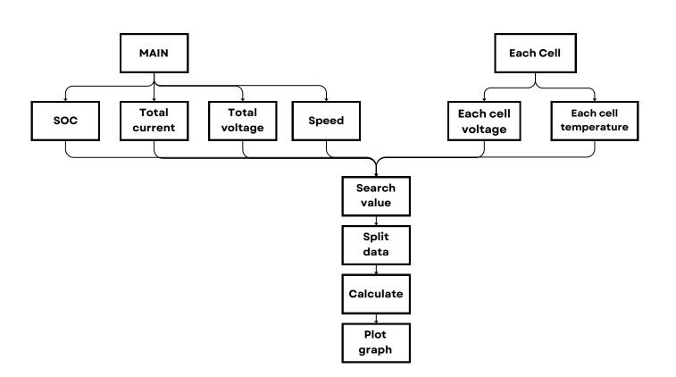
This is the diagram of the system. First, it reads a CSV message log file. The main part has SOC, Total current, Total Voltage, and speed to be displayed. The each cell part has voltages of 156 cells and temperatures of 32 positions. Then, the program searches for the specified ID, splits the data into individual bytes, calculates the data, and plots the graph.
