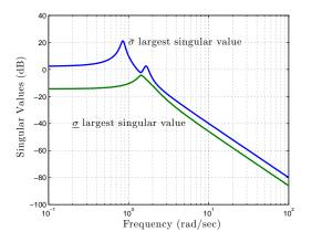
An example of the singular value plot of a mass-spring-damper system, using a command sigma.
