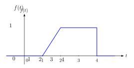
Find the Laplace Transform of f(t) depicted in Figure above. The signal can be described as
