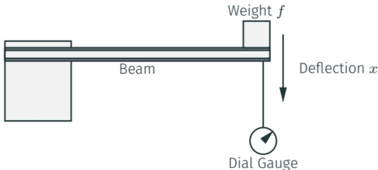
The deflection of a cantilever beam is the distance its end moves in response to a force applied at the end. The following table gives the measured deflection  $x$  that was produced in a particular beam by the given applied force  $f$ .
