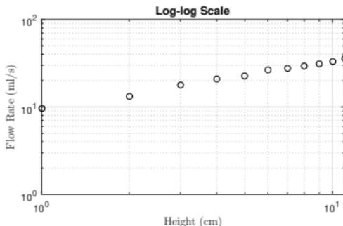
The log-log plot shown that the data lie close to a straight line, so we can use the power function to describe the flow rate as a function of height. Thus we can write
