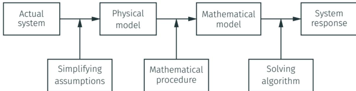
Flow in a Process Connecting an Actual Dynamic System to Its Response
