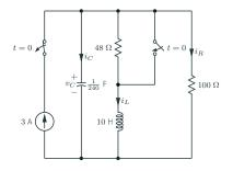
At t<0 , capacitor acts as an open circuit, and inductor acts as a short circuit.
