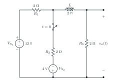
The switch in the network opens at t = 0. Let us find the output voltage  $v_o(t)$  for t > 0.
